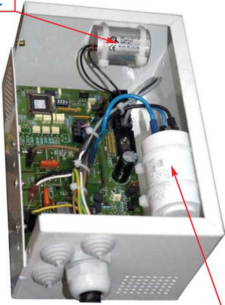
**RUNNING CAPACITOR ROTARY COMPRESSOR**
