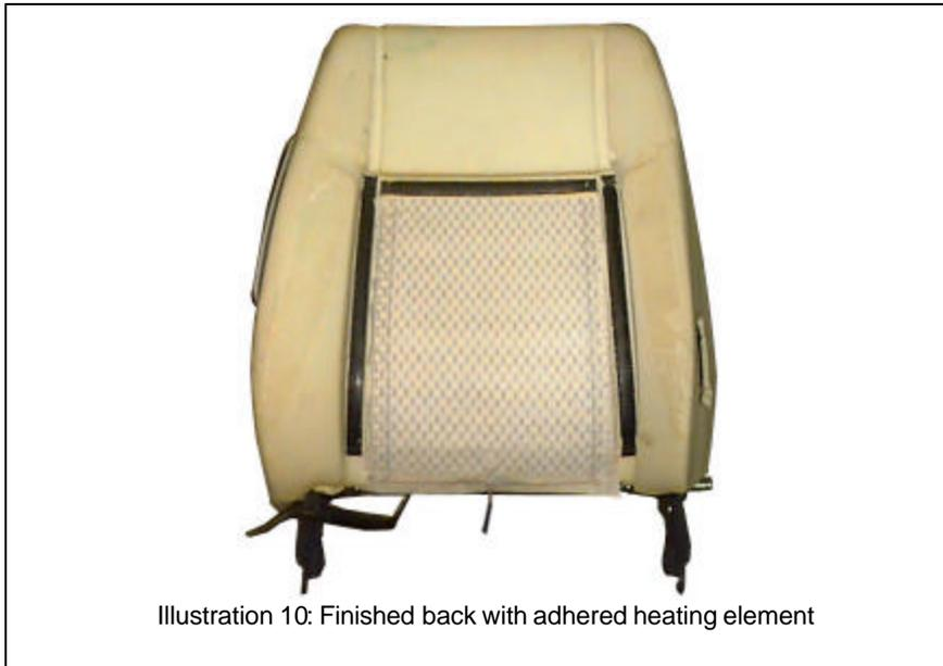
Illustration 10: Finished back with adhered heating element
