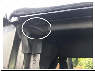
Foam installed and ThrowBack re-installed on vehicle.
