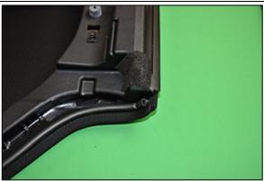
Wrap the foam around the frame and. Be sure seams are closed to prevent water leaks.
