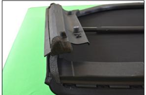
The foam section should cover the end cap of the front rail and wrap around to the upper side of the rail
