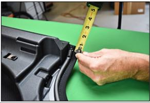
Start and terminate the new seal approximately 3/4" from the edge of the roof. This is to prevent it from showing from the outside of the vehicle. Press the gasket to the plastic strip firmly as you go.
