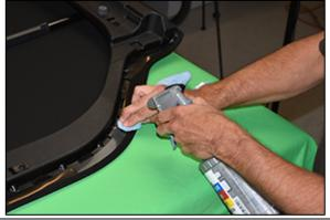
Prep the plastic edge of the fabric with wax and grease remover.
