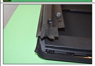
Following the contour of the ThrowBack frame, adhere the foam to the frame but do not wrap the foam around the frame at this time.
