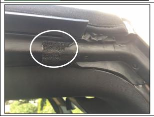
Foam installed and ThrowBack re-installed on vehicle.
