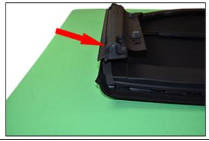
Remove ThrowBack top and turn upside down on bench before proceeding. Remove factory foam as shown in adjacent picture from both front corners.
