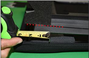
After cleaning the area with wax and grease remover, align the outside edge of the front foam piece with the inside of the groove on the frame. The rear edge of the foam is aligned approximately 1.5 in. from the front edge of the frame.
