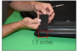
Remove ThrowBack top and turn upside down on bench before proceeding. Align the outside edge of the foam on the inside edge of the groove in the frame as shown.
